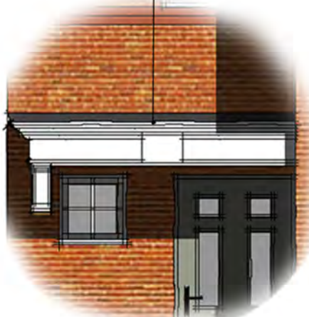
Flat portico with wood grain and rolled lead effect top. Individual formal 6 panel styled front door with ironmongery letterbox.
